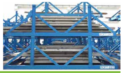
Transport Rack Slab
